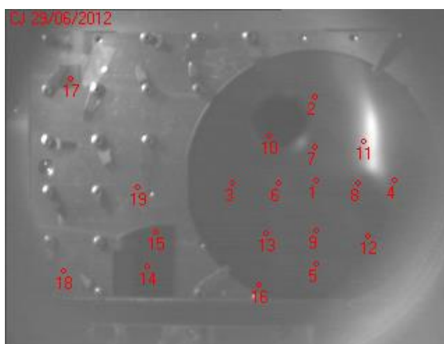
Figure 13: RBS typically measured at 13 locations across the As implanted QA wafer.
