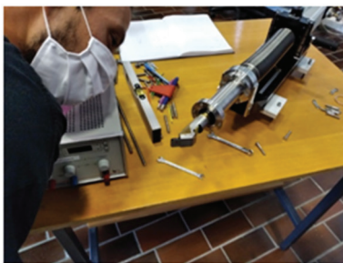
The detector outside the chamber (left) and the “head” of the detector is bent to 45° to fit into the existing chamber (right) Photos: © JSI
