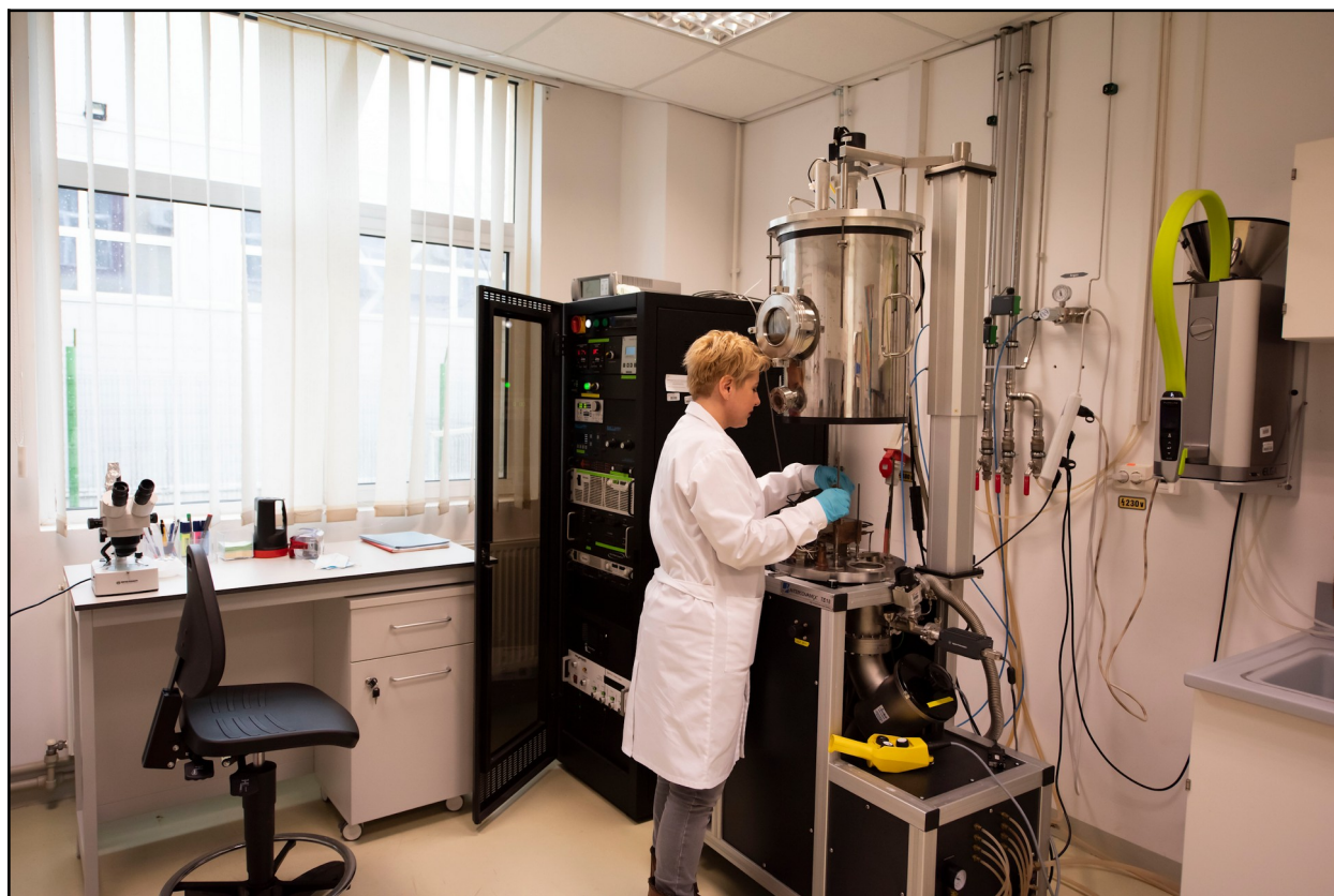
1. TE18-High Vacuum Deposition System produced by Intercovamex Company
