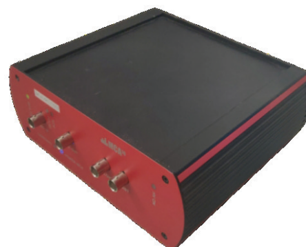
Multi Channel Analyzer MCA 16 developed at Józef Stefan Institute © JSI
